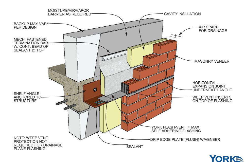
SHELF ANGLE DETAIL YORK FLASH-VENT™ MAX SELF ADHERING FLASHING W/ DRIP EDGE
