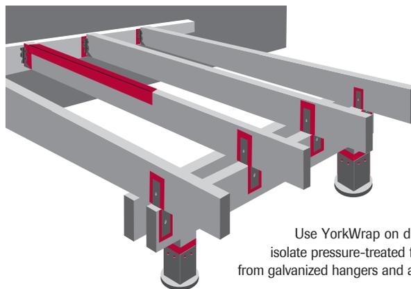
Use YorkWrap on decks to isolate pressure-treated framing from galvanized hangers and anchors
